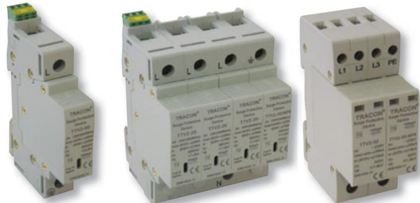
The type 2 surge arresters are applicable to discharge overvoltage caused by switch-type (8/20μs wave-form) over currents.
